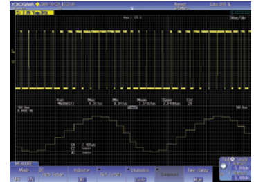
Trend display of waveform parameters Histogram display using the time axis
